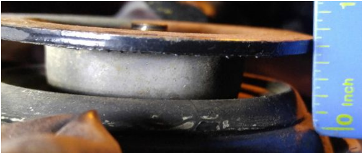
COLLAPSED SHOCK MOUNT CLOSE-UP
