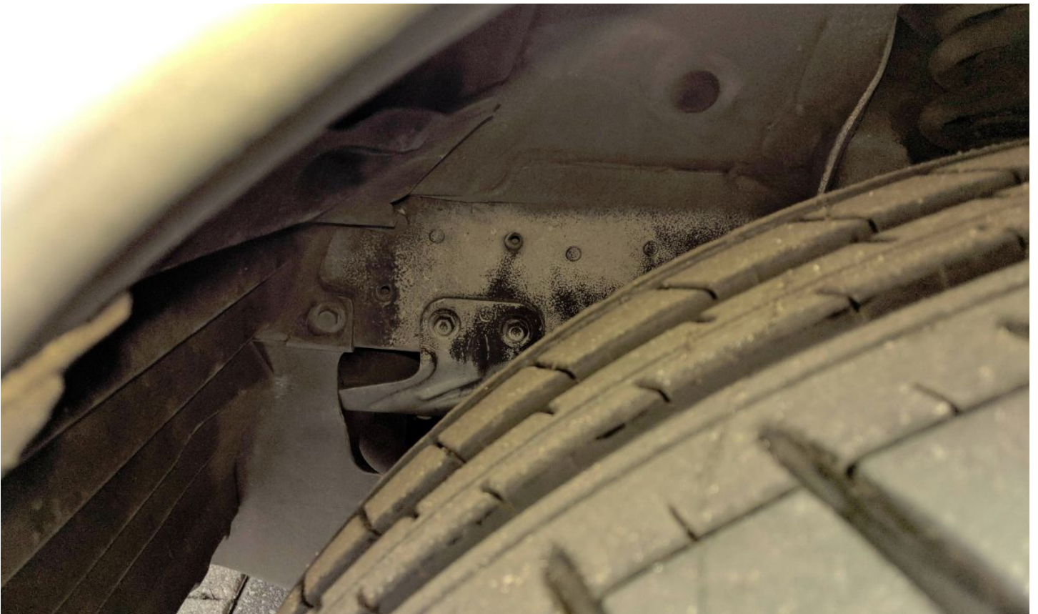
NB FRAME RAIL INTACT (NO RUST)
