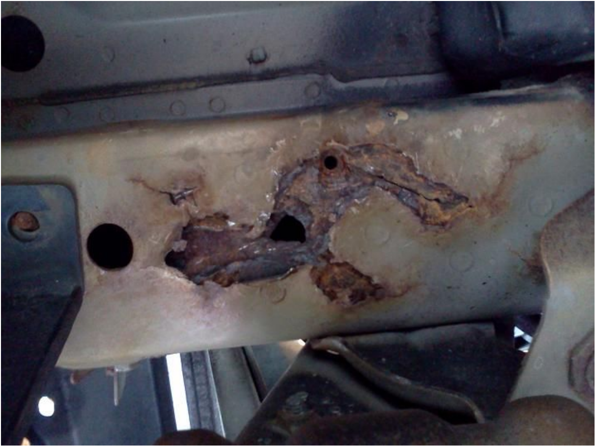
NB FRAME RAIL RUST
